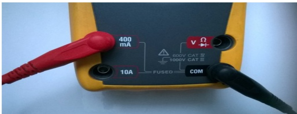
Test leads and sockets on a DMM, setup to measure current | Source
